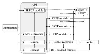
Fig. 2. Software architecture of uvgRTP.
