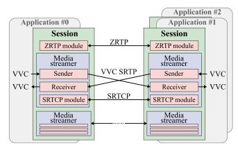
Fig. 1. uvgRTP usage scenario for streaming encrypted VVC.
