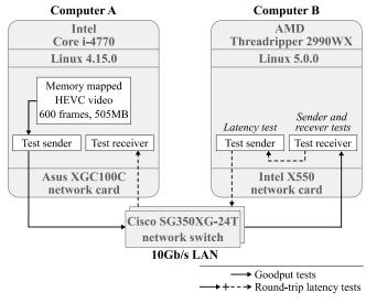
Fig. 5. Experimental setup.
