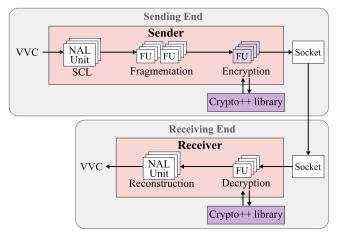
Fig. 4. The E2EE workflow for VVC video streaming in uvgRTP.
