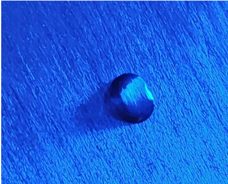
Figure 36. Water droplet on A Hard treated surface, droplet length 3mm
