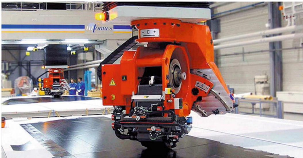
Figure 6. TORRESLAYUP ATL machine with 11 axes of movement (10)
