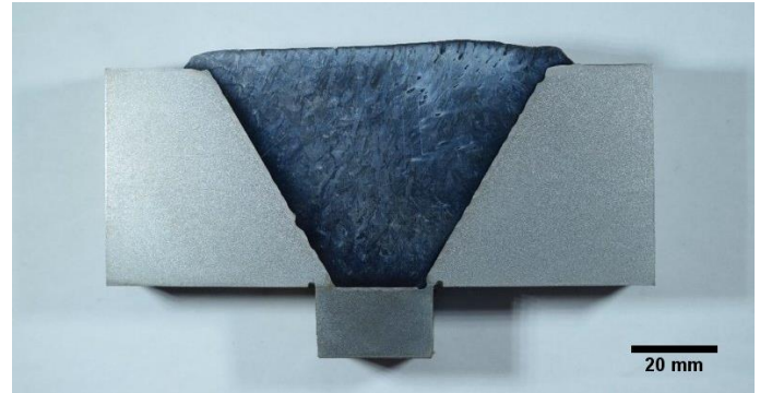
FIG. 2. CROSS-SECTION OF THE MOCK-UP WELD AFTER POLISHING. SEE FIG 1 FOR THE WELD PASS LAYOUT, DIMENSIONS AND MATERIALS.
