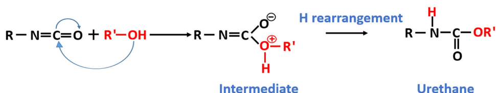
Figure 3: Reaction of an isocyanate with alcohol.
