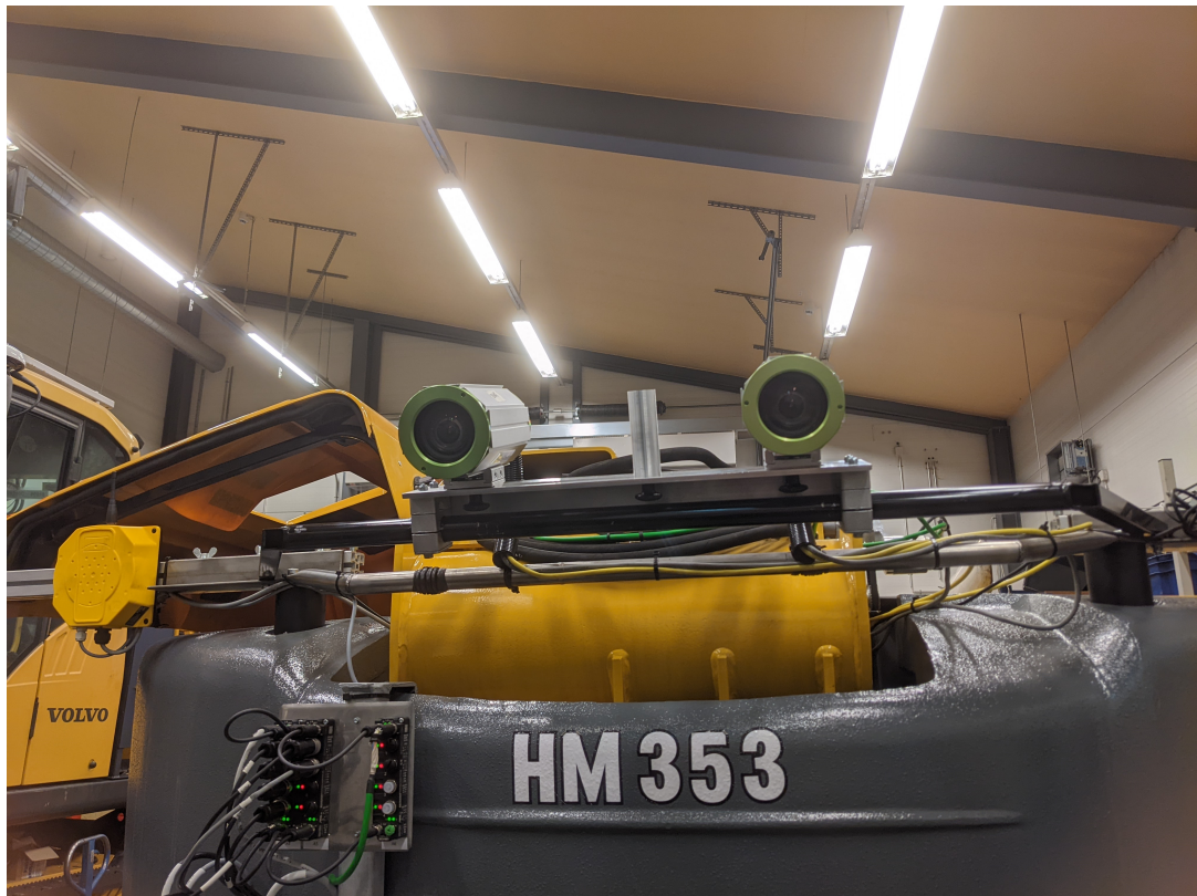
Figure 17. Photograph of the Basler stereo cameras inside casings in stereo setup mounted onto a steel frame.
