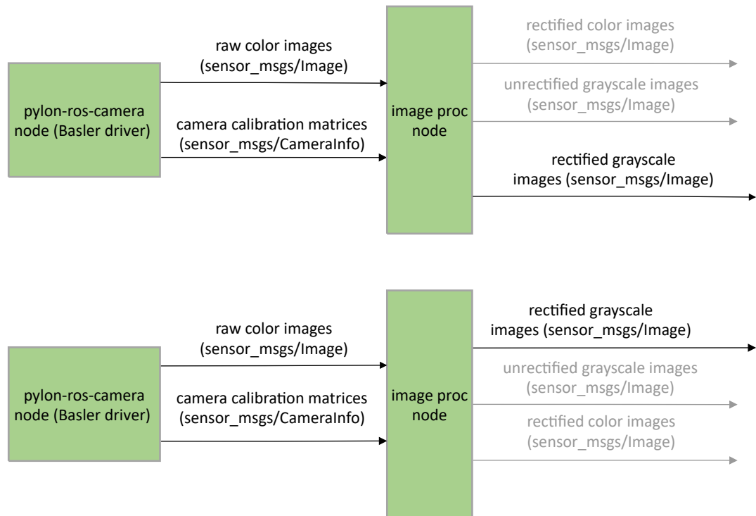
Figure 25. Image undistortion and rectification part of the 3D perception system ROS architecture.
