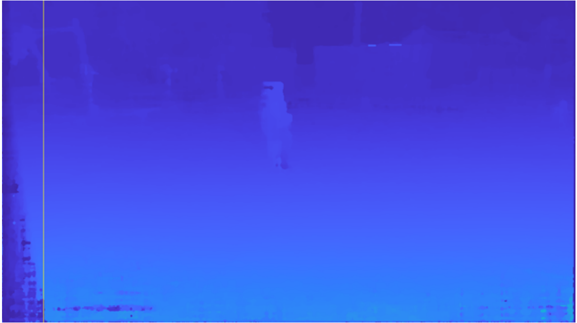
Figure 28. Example disparity image showing the segmented area on the left of the white line. A colourmap has been applied to the disparity for better visualisation.
