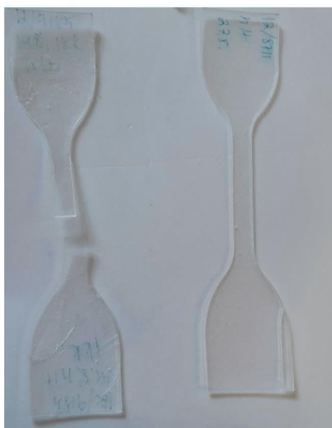
Fig. ESI 1. Tensile strength specimen and the typical breaking point (CC-HDI-S + A-PEI-3).
