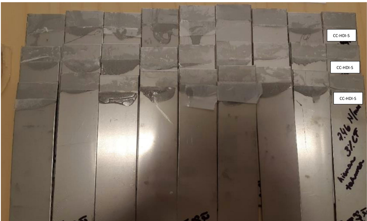
Fig. ESI 3. Lap shear strength specimen on stainless steel, failure type adhesive (CC-HDI-S+ A-PEI-1, A-PEI-2 and A-PEI-3).
