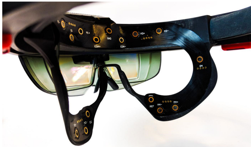
Figure 6. PhysioHMD records physiological data through the contact with the skin (credit: Guillermo Bernal, https://www.media.mit.edu/projects/physiohmd/overview/ , accessed on 1 December 2021, image cropped).
