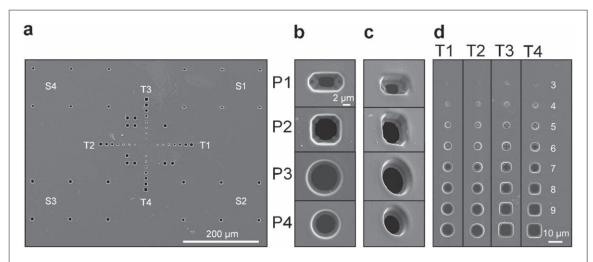
**Figure 3.** (a) A SEM image of a quality control test pattern in the middle of a fabricated membrane and the corners of the opening grids. (b) SEM images of the openings from the top. (c) The openings seen from an angle. (d) Magnified images of the test sites (T1-T4) of the quality control pattern. The pores pass through the membrane when the size of the pore design is at least 7  $\mu$ m.
