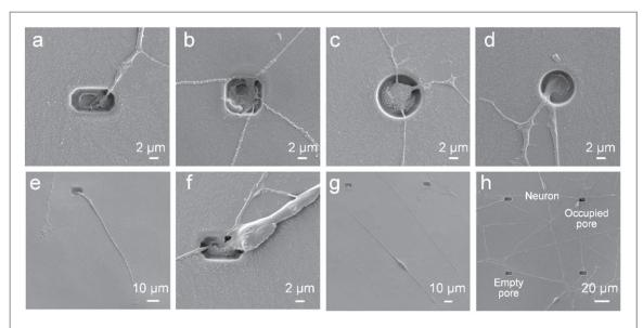
Figure 5. Detailed SEM images of neurites on the bottom side of the membrane. (a)–(d) Examples of the neurites in each tested pore types (P1-P4) at DIV1. (e) A neurite protruding through the membrane from the seeding side to the opposite side of the membrane (DIV1). (f) An example of a neuron migrating through the opening at DIV1. (g) Unconnected neuron on the bottom side of the membrane (DIV1). (h) Neurite network on bottom of the mebrane at DIV7.
