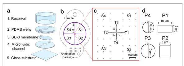
**Figure 1.** (a) Exploded view of the microfluidic cell culture device with description of each part. (b) The SU-8 membrane was divided into four test sectors each containing one pore type. (c) The pores were placed in the sectors in grid formations with  $100~\mu m$  separation. In addition, there was a quality control test pattern in the middle of the membrane. (d) The dimensions of the designed pores.
