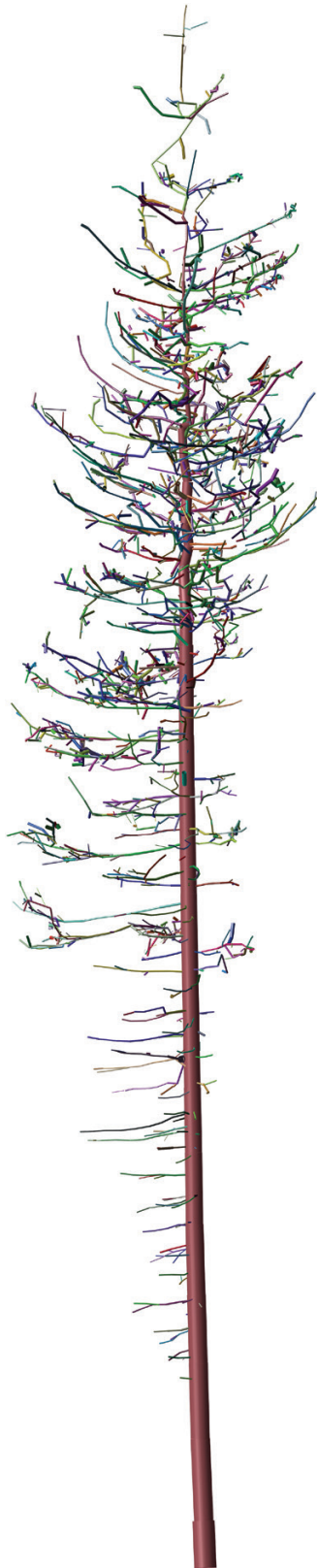
FIG. 4. Example of a quantitative structural model (QSM). QSMs are vital for extracting detailed structural measurements of woody plants useful in downstream analysis such as FSPM input or validation and calibration. Cylinders are used to reconstruct 3-D structure from point cloud data. Here, the different colours represent the different branches of the tree.
