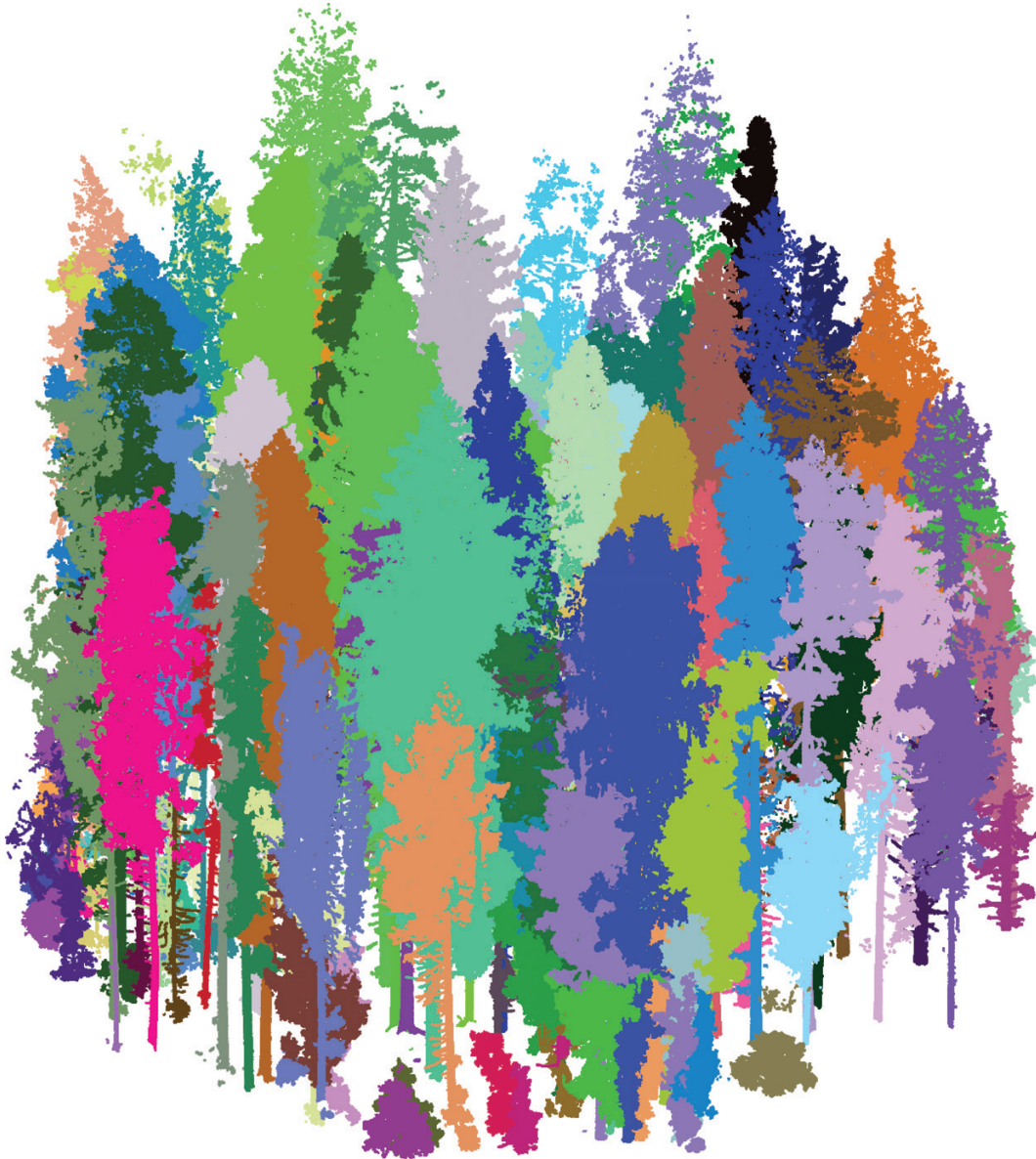
FIG. 5. Segmentation of individual trees from a whole-forest scan. Although manual segmentation is possible, automation or semi-automation of this process can greatly speed up the processing of TLS data. The different colours delineate between individual trees in the forest community.
