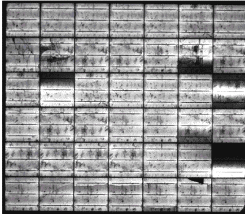
Figure 3.9. EL image of PV module with broken interconnect ribbons [25].
