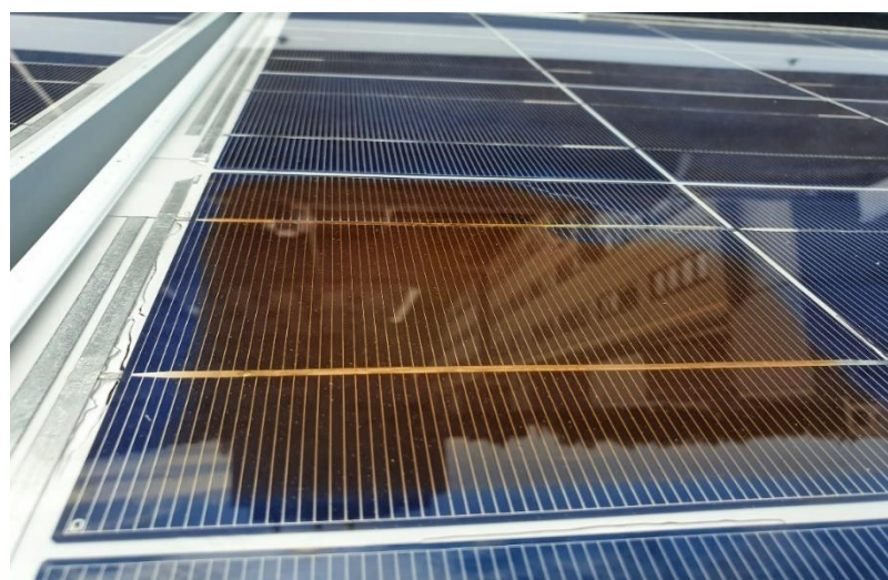
Figure 5.21. EVA discoloration in a single PV cell.
