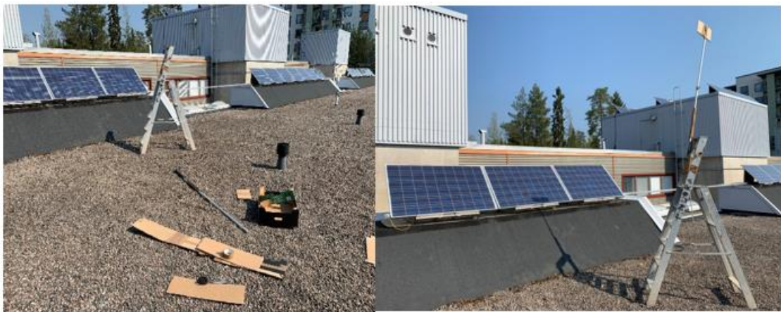
Figure 5.11. an artificial partial shadow on two adjacent PV cells.
