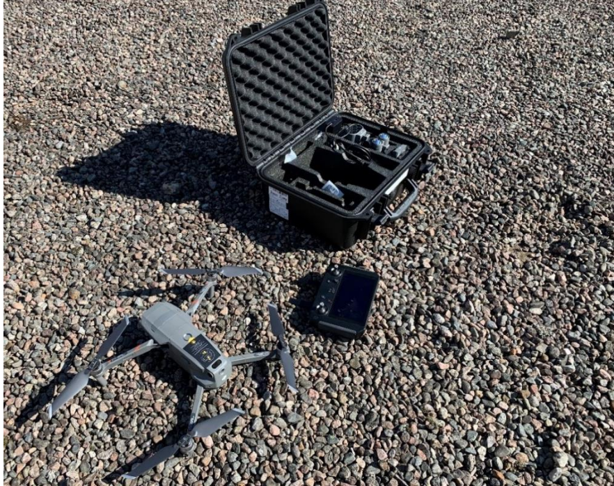
Figure 5.1. DJI Mavic 2 Enterprise Dual its visual and thermal cameras, flight controller, battery charger, and additional accessories.
