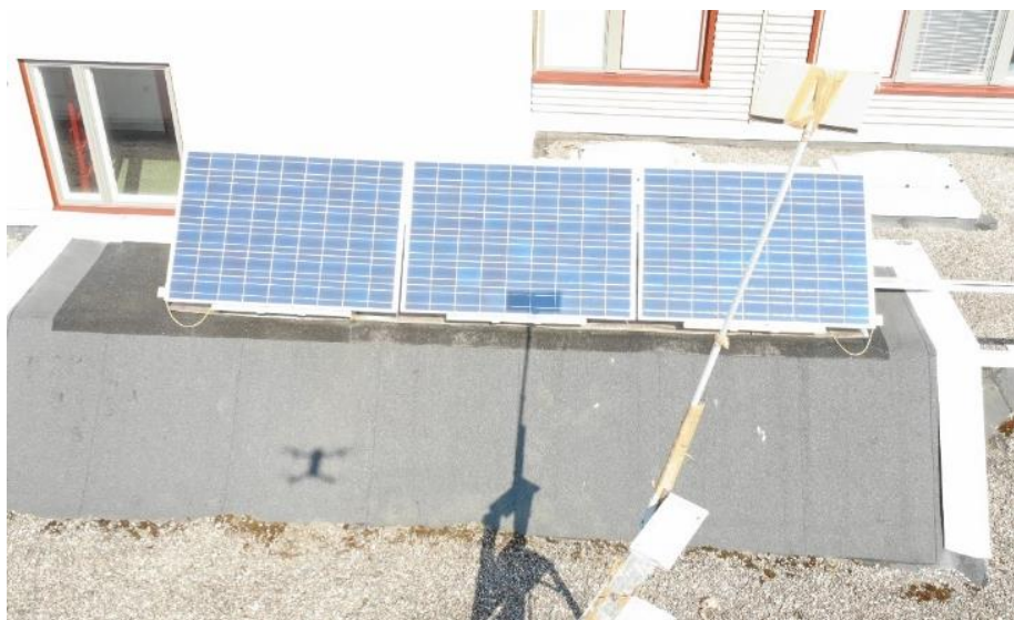
Figure 5.12. Visual image of an artificial shadow on two contiguous PV cells.
