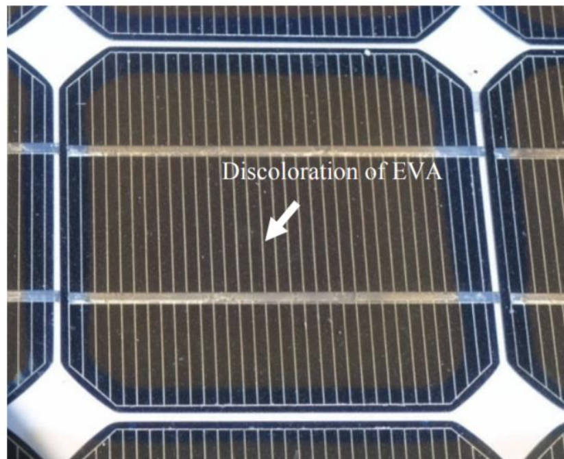
Figure 3.7. EVA discoloration of aged Monocrystalline PV module [43].
