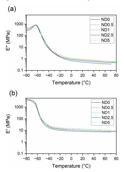
Figure 5. The effect of partial replacement of CB by NDs on (a) storage modulus, (b) loss modulus.
