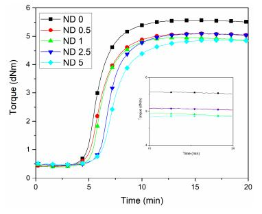
Figure 1. Rheometric curves of NR/BR compounds at different ND/CB concentrations.
