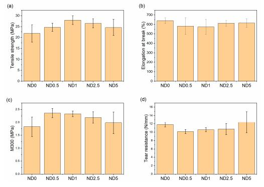
**Figure 3.** The effect of NDs on the mechanical properties (**a**) tensile strength, (**b**) elongation at break, (**c**) 300% modulus, and (**d**) tear resistance.
