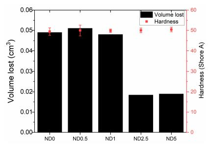
Figure 4. Wear resistance of ND-CB filled rubber compound.
