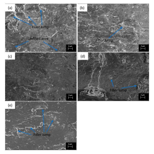
**Figure 2.** SEM images from the fracture surface (tensile test) of the compounds (**a**) ND0, (**b**) ND0.5, (**c**) ND1, (**d**) ND2.5, (**e**) ND5.
