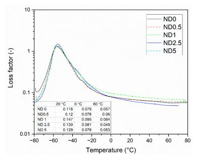
Figure 6. The loss factor of the rubber compounds as a function of temperature.
