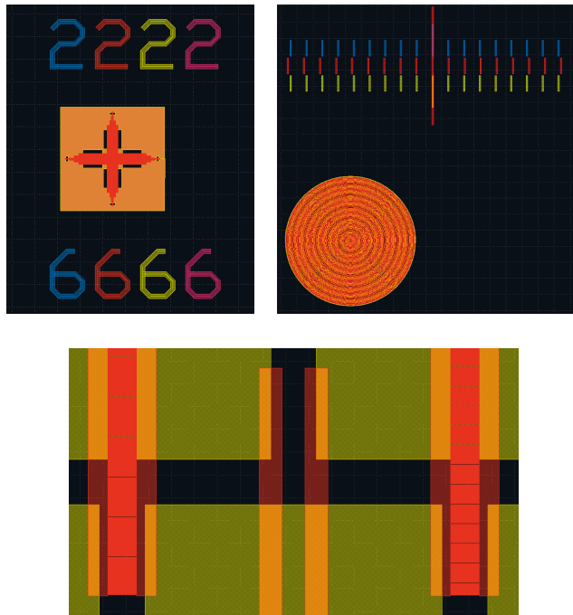
Fig. 3.6 The mask pictures are not to scale relative to each other. Top left: Row and column numbers next to alignment markers on each mask layer. Masks often have (partial) translational symmetry on some layers, and sometimes alignment markers from a wrong row or column might be used accidentally in device processing, resulting in the failure of the outermost components on the mask or even the whole wafer. Indexing the alignment markers prevents this kind of mistake. Top right: Vernier scale and Moiré rings on mask layers to increase alignment accuracy. The success of these approaches was not tested conclusively. Bottom: Border between two adjacent component bars on the mask. NIL layer shown in red, metallization layer shown in yellow. The bars can be separated by cleaving anywhere between the top and bottom metals, and the overlap between the DBR grating (top bar) and RWG (bottom bar) ensures that both bars remain functional. This way a wasted spacer region of about 500\ \mu\text{m} can be avoided between adjacent bars.
