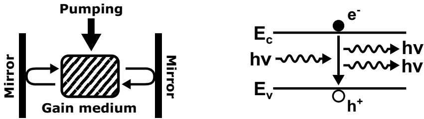
Fig. 2.1 Left: Schematic model of a laser. Light circulates between the mirrors and is amplified through stimulated emission by the gain medium. The amplification is made possible by the excitation of the medium through pumping. Right: Stimulated emission in semiconductor. Excited electron e^- recombines with the hole h^+ when an incident photon with energy h\nu interacts with the system. As a result a new photon with identical energy, phase, and direction is generated.
