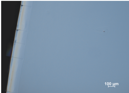
(a) Bare semiconductor membrane after the substrate-removal, single-side bonded onto SiC.
