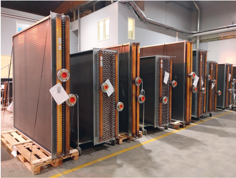
Fig. 1. Illustration of different sizes of fin-and-tube heat exchangers.
