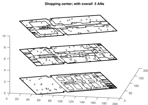
Fig. 1. The building map used in the simulator. Red circles show examples of AN location and blue crosses show examples of robot locations
