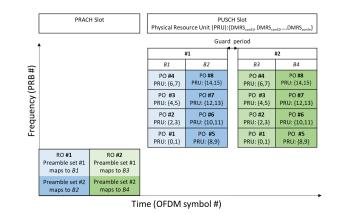
Fig. 2: Example of the mapping between the preamble in the RACH occasion (RO) and the physical resource unit (PRU) in the PUSCH occasion (PO) of MsgA in two-step RACH procedure
