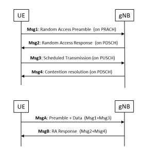
Fig. 1: Random access procedures operation in four-step RACH (top) and two-step RACH (bottom)
