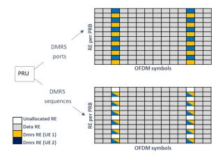
Fig. 3: Slot configuration example of a MsgA payload transmission from 2UEs within the same PO. PRU: {DMRS $_{conf1}$ , DMRS $_{conf2}$ }, associated with two different DMRS ports (top) or two different DMRS sequences (bottom).
