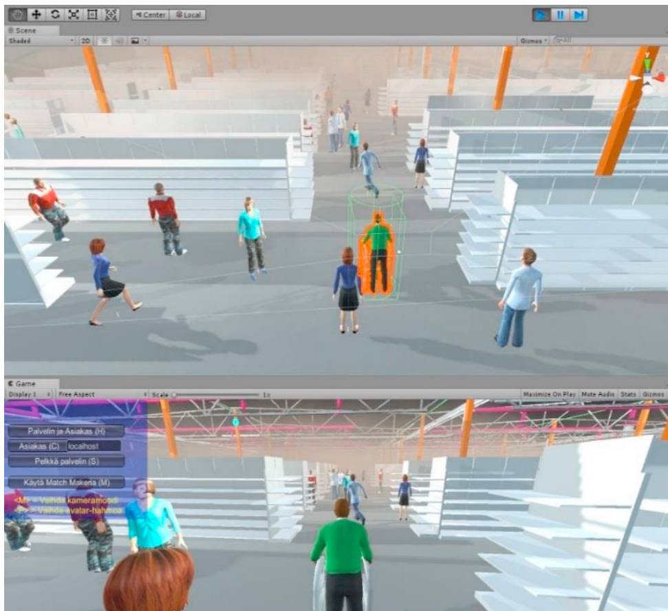
Fig. 1. A simulation application realized with the Unity game engine. A game collider corresponding to the spatial need of a game character is visible in the figure.
