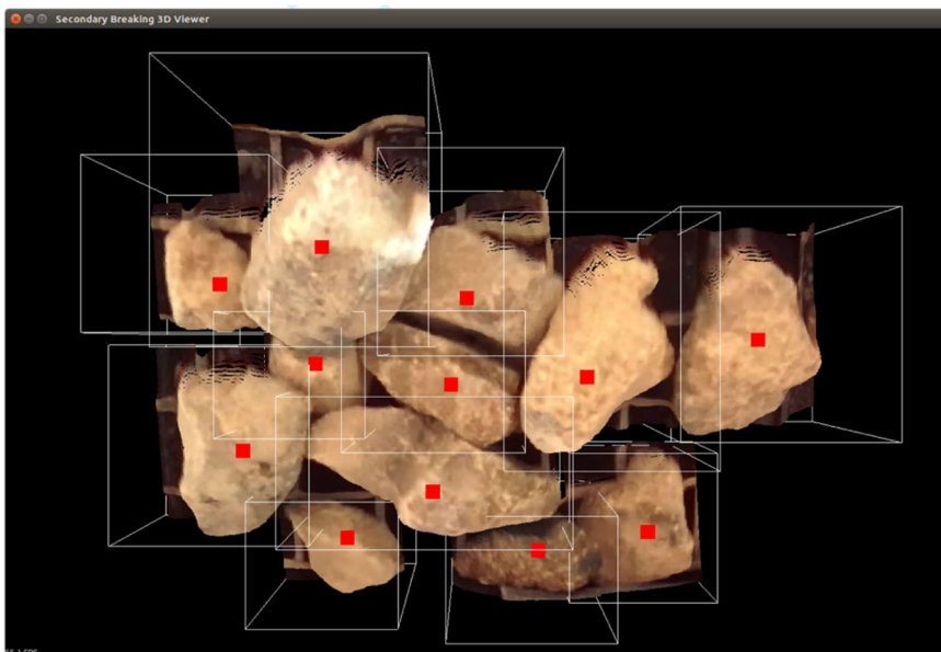
FIGURE 23 Real-time view of the detected rocks with breaking positions indicated in red dots [Color figure can be viewed at wileyonlinelibrary.com ]
