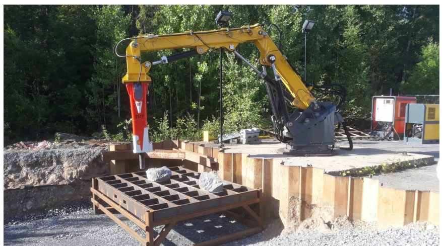
FIGURE 3 Rambooms X88-540R breaker boom at the field test site at Tampere University [Color figure can be viewed at wileyonlinelibrary.com ]
