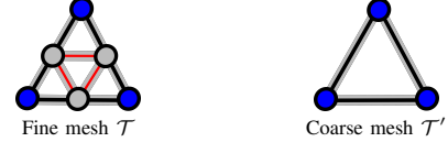
Fig. 3. A schematic illustration of the nested mesh structure. The fine mesh \mathcal{T} (left) is used in the forward simulation and the coarse mesh, \mathcal{T}' (right) in the inversion.
