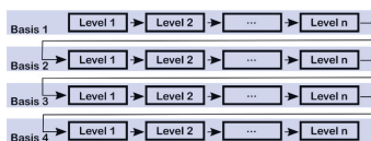
Fig. 4. A schematic visualization of the data flow in the randomized multiresolution scan. The average of the MAP estimates obtained for the k -th multiresolution decomposition is used as the initial guess for the k + 1 -th one.
