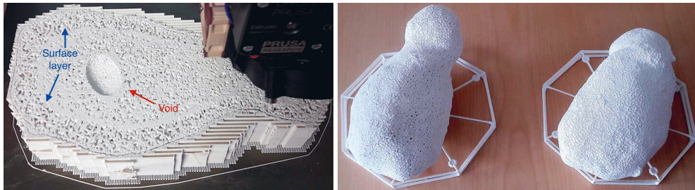
Figure 3.4 Analogue interior structure during the 3D printing process (left) and the final object on the support plate (right). The mantle and the void structures are clearly visible during the additive manufacturing process. During the printing process, the object is surrounded by a support structure which is removed after the printing. The different filling levels of the surface layer and the interior around the void are clearly visible, as is the inflated edge structure. The surface of the final object is fairly smooth despite the wireframe structure being clearly visible. Photos: Sampsa Pursiainen.
