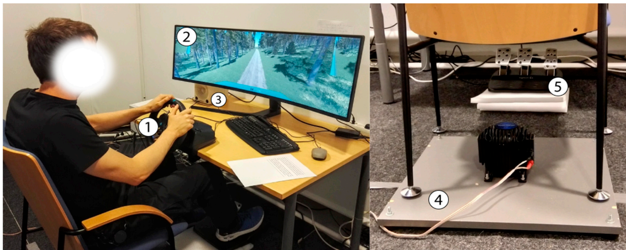
Figure 1. Multimodal driving simulator set-up: 1 and 5—Logitech G29 Driving Force wheel and pedals, 2—49" curved display, 3—speaker, and 4—Buttkicker LFE.
