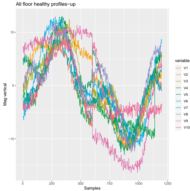
Figure 5. Profiles from healthy rides (The figure shows first 10 rides from the combined version of elevator start and stop events from magnetic signals in z-direction i.e., Mag vertical. Equal number of profiles as in Figure 4 are extracted from all floor combinations before the time period of fault occurred in upward movement of elevator system. Color labelling is based on number of rides available in the data during this time period i.e., variable.).
