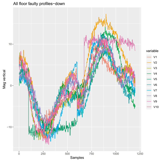
Figure 8. Profiles from faulty rides (similar to Figure 4 but in downward movement of elevator system).
