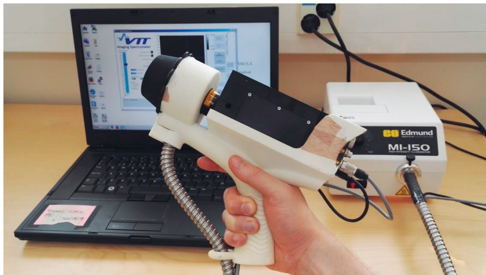
Figure 11. A handheld prototype of hyperspectral camera used in Study III. The camera is connected to a laptop with the image acquisition software. On the right side of the laptop is a broadband halogen light source which is connected to the camera via optical fibre. Photo by author.
