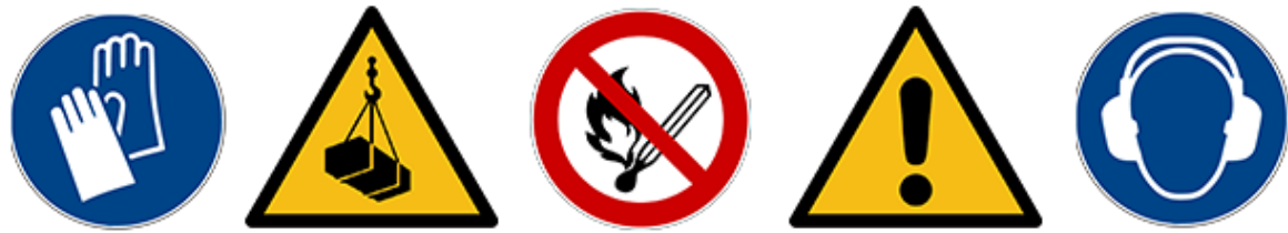
Figure 7. Safety signs used at KONE [ISO 7010, 2019].
