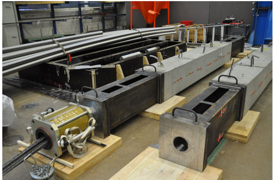
FIGURE 2 Test beams with hollow cylinder jack assembled on active end of the beam
