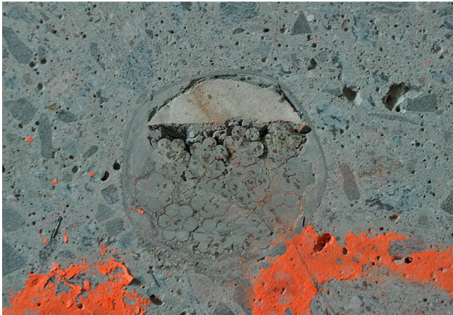
FIGURE 5 Strand layout in tendon duct, arrangements for void in test and effective perimeters for tendon
