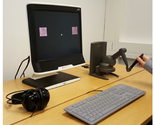
Figure 3: The experiment setup involved a Tobii T60 gaze tracker and a Phantom force-feedback device. The two skin models on the screen have the medium size of 4.8 cm (out of the three size levels) and the large distance of 24.3 cm between them (out of the three distance levels).
