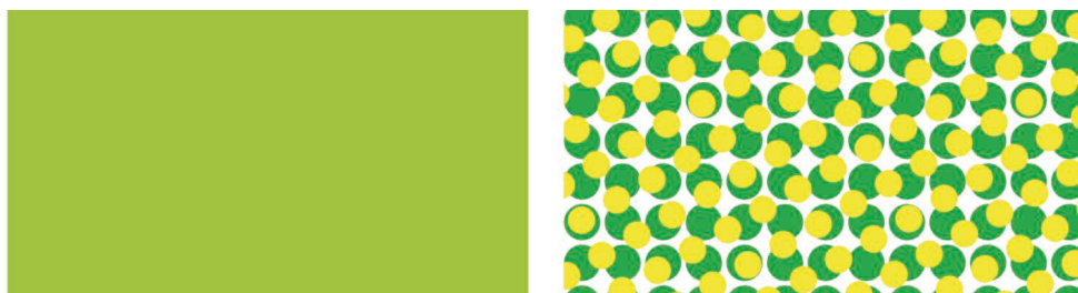
Figure 42 Full coverage spot color vs. halftone screening of process colors (K. Lankinen)
