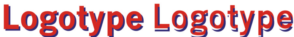
Figure 37 Sample of correct and incorrect registration of a two-color print (K. Lankinen)
