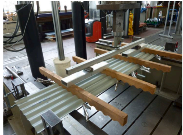
Fig. 5. Single span tests: SSP-18-100-1.
