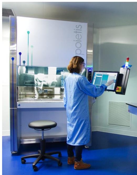
Figure 10. A 3D bioprinter based on laser-assisted method is bulky and non-transportable compared to extrusion or inkjet-based printers. [40]
