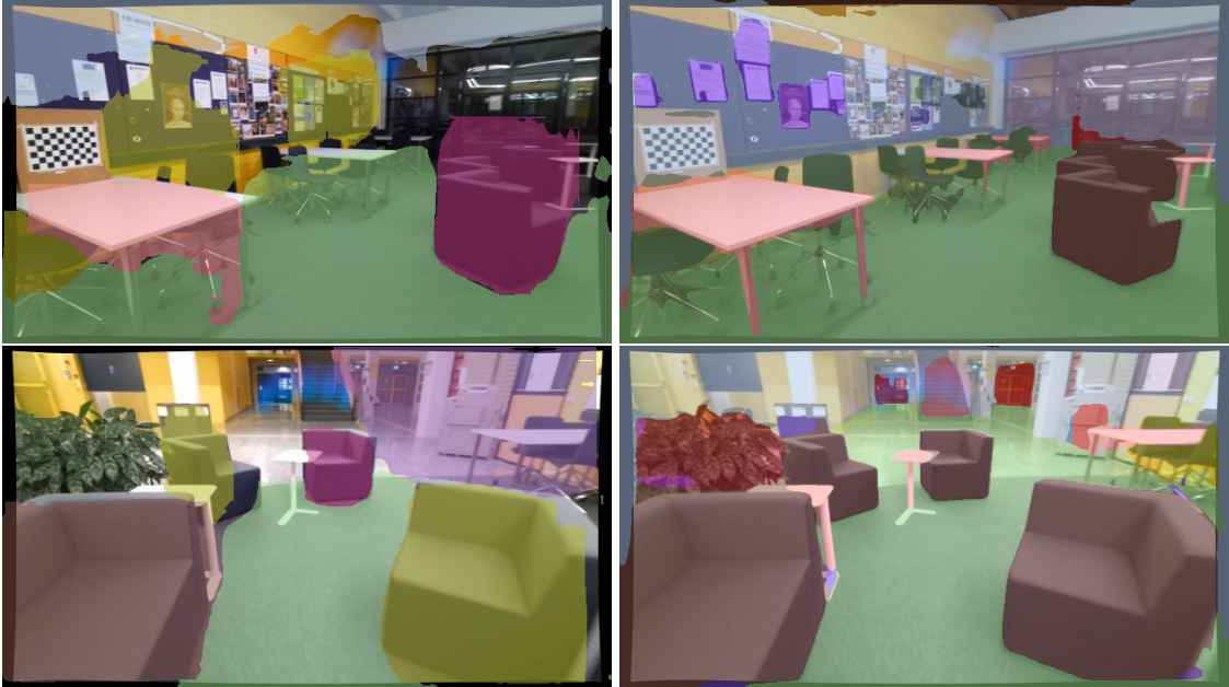
(a) EfficientPS panoptic segmentation
