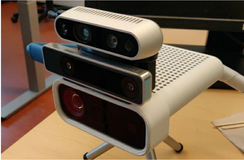
Figure 4.1. The camera system used for indoor reconstruction. From top to bottom: Intel Realsense D435i RGB-D camera, Intel Realsense T265 tracking camera, Microsoft Azure Kinect RGB-D camera.
