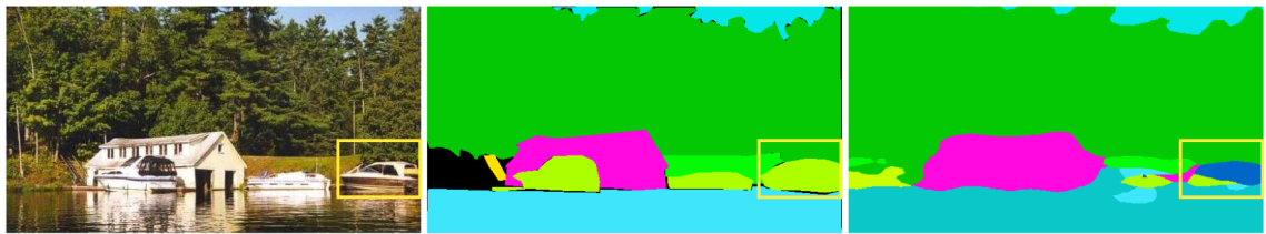
Figure 2.10. An example in [89]. Left: original image, middle: ground-truth, right: FCN prediction. A boat (labeled as light green) is misclassified as a car (blue) due to missing the global context: a boat is much more likely to be found in a river.
