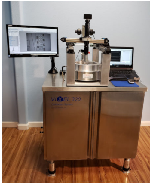
Figure 3.3. VIXEL-320 wet thermal oxidation furnace by California Scientific [19].
