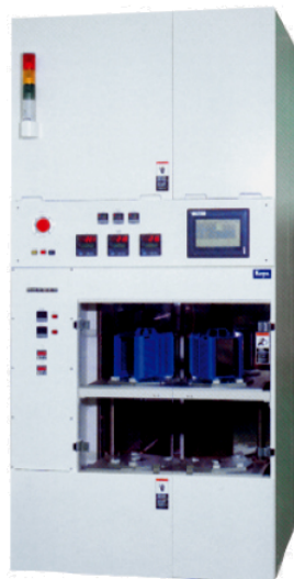
Figure 3.4. VF-3000 vertical furnace by Koyo Thermo Systems [20].
