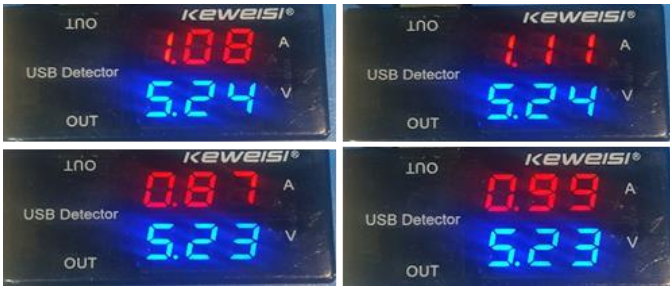
Fig. 15. Power consumption for on-board execution of deep learning model on Raspberry Pi. The upper value shows current while the second value shows voltage consumed by the Raspberry Pi during execution of the DNN model.
