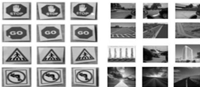
Fig. 9. Training of Haar cascades with Positive (left) and Negative (right) images for a traffic signs detection.
