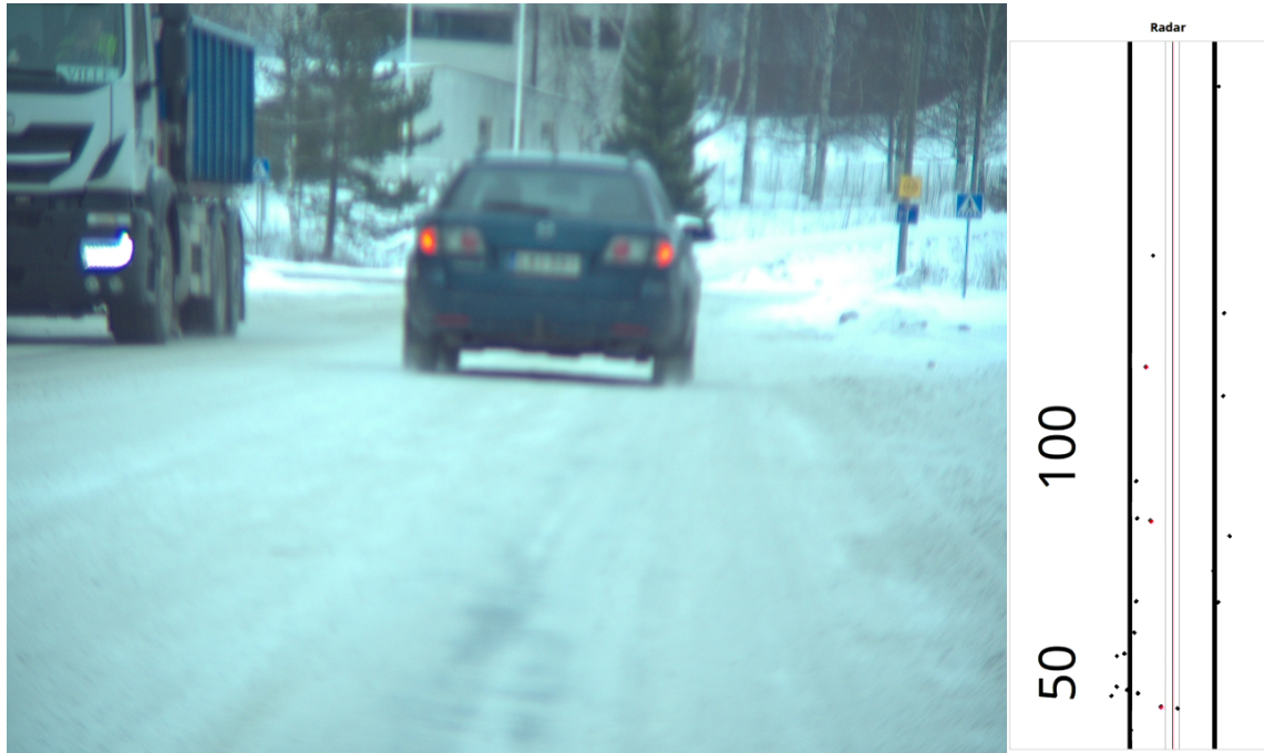
Figure 6.5. Two oncoming vehicles in different lanes. The one on the left side is considered as an obstacle 46 meters away.
