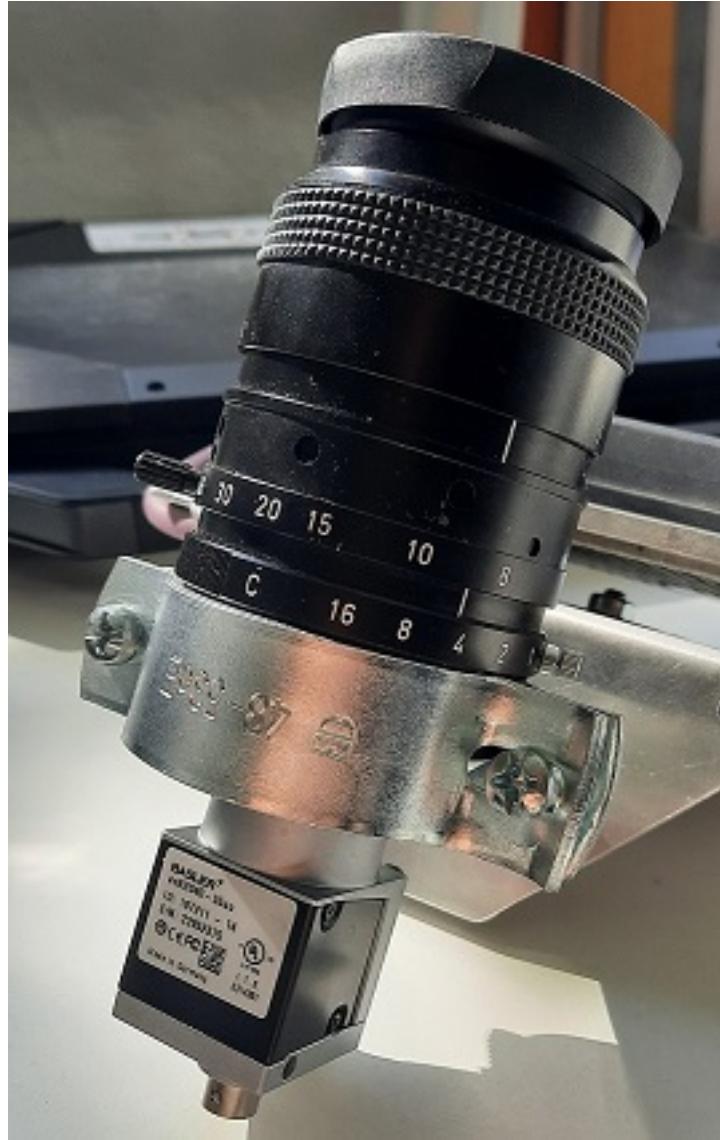
Figure 5.7. Basler RGB camera with attached Canon zoom lens.
