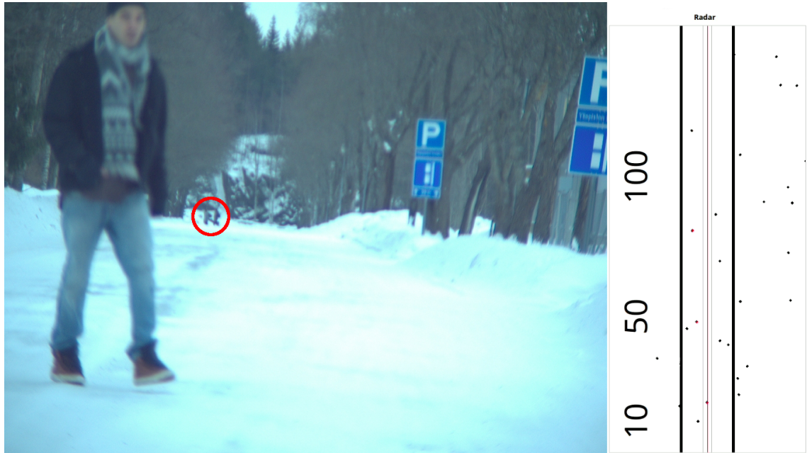
Figure 6.7. Nearby person is detected as an obstacle, but two people on the crossing sidewalk are not detected. The radar is showing constant detections 3.8 to 5.6 meters on the left, that are probably snow banks or light poles.
