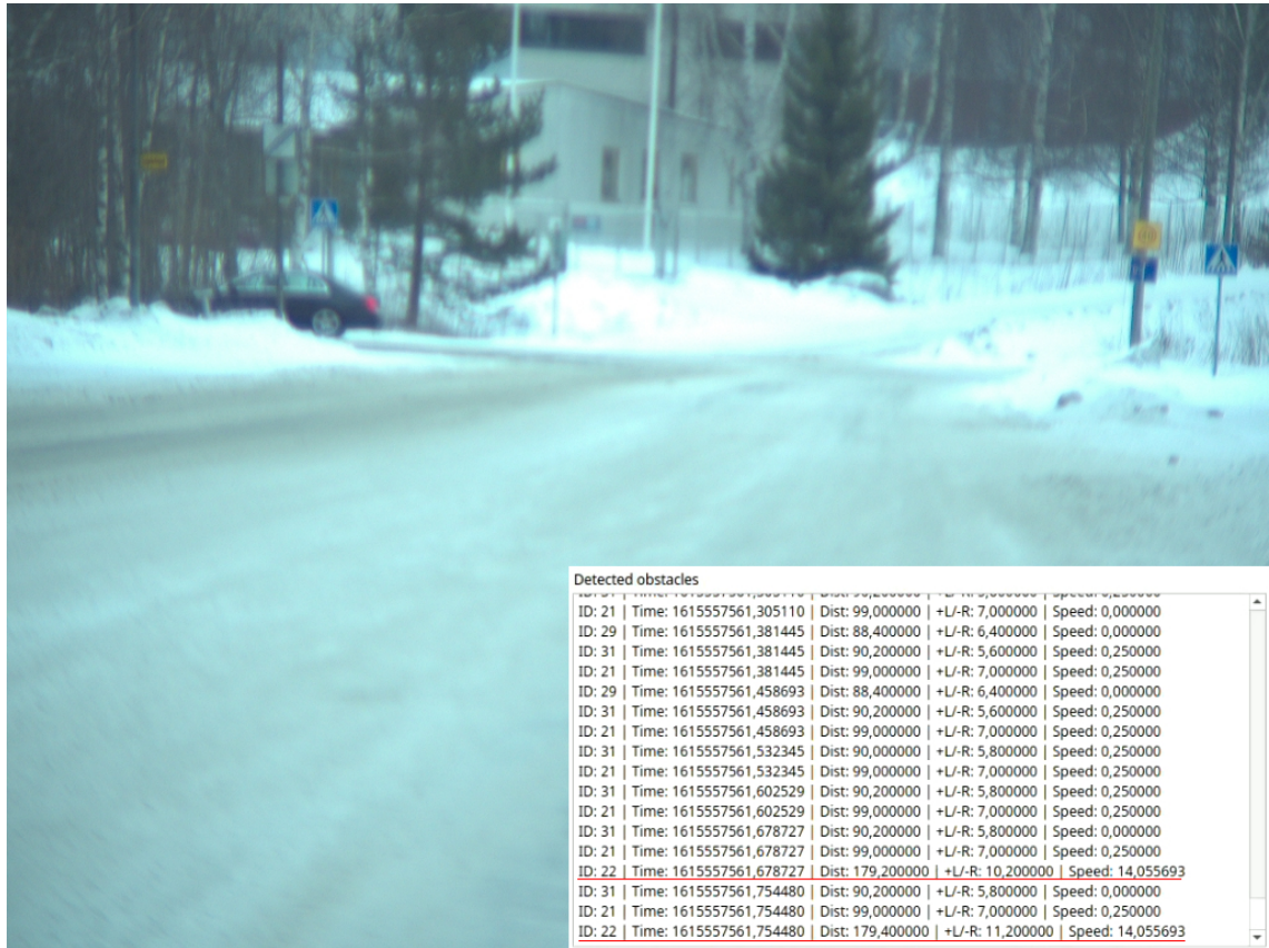
Figure 6.6. Moving vehicle detected at a distance of approximately 179 meters. Its velocity is measured in meters per second. Here the "Dist" is the distance from the sensor straight to the trajectory that the vehicle is running on, and "+L/-R" denotes how many meters left or right the detection is from this point. (x/y in Fig. 5.4)
