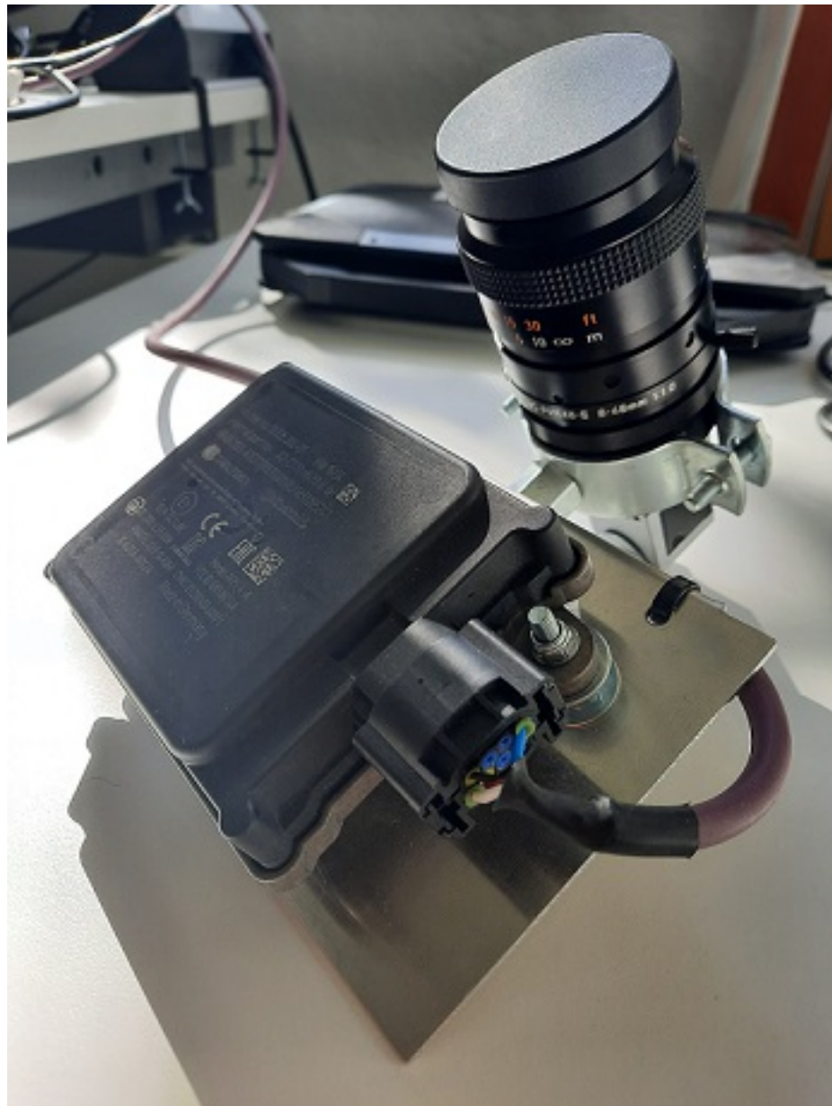
Figure 5.3. Continental ARS 408-21 SC1 radar and Basler acA2040-55uc RGB camera attached together to ensure same directivity.
