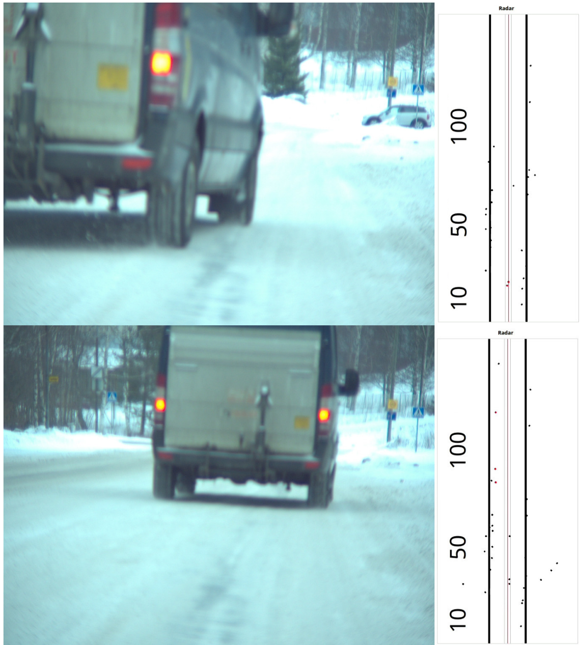
Figure 6.4. In upper scene, the van is detected to be an obstacle 21.6 meters away, whereas in the lower scene where the van has moved slightly to the right, it is categorized to be outside of the tracks.
