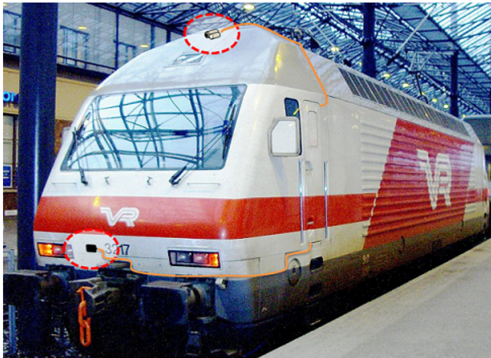
Figure 1.1. The radar is located on the bumper whereas the cameras as well as GNSS antenna are on the roof, above the windshield. The computer for data processing sits in the cockpit along with system's powering equipment. Photo: Courtesy of Pertti Peussa.
