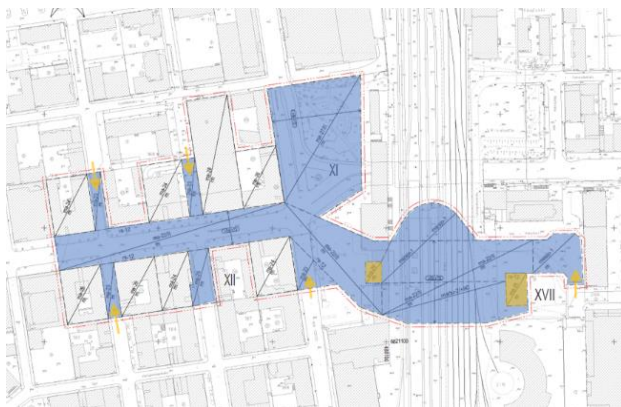
The two-story underground parking and facilities accessible from the streets and neighbor buildings basements. The drive-ins are shown with arrows and other staircases and elevator access shafts with yellow blocks. Source: Kartat.tampere.fi
