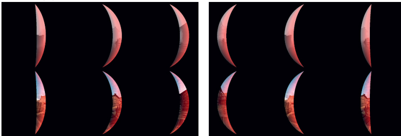
(e) Seam stitching and blending for both depth maps (top row) and RGB values (bottom row). The final pixel will either be a forward warp pixel, backward pixel, or a blend of both warps.
