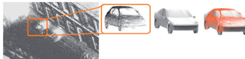
(b) Example of a 3D car model fitted and rendered to a point cloud
