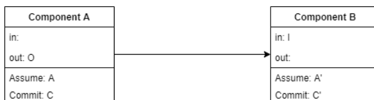
Figure 1. System of two components connected by their interfaces. [Gruhn and Rüdiger 2018, Ch. 1]
