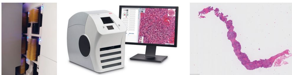
Figure 1.1 Microscopy slides (left), Aperio scanner 1 (center), a WSI of a prostate biopsy (right).
