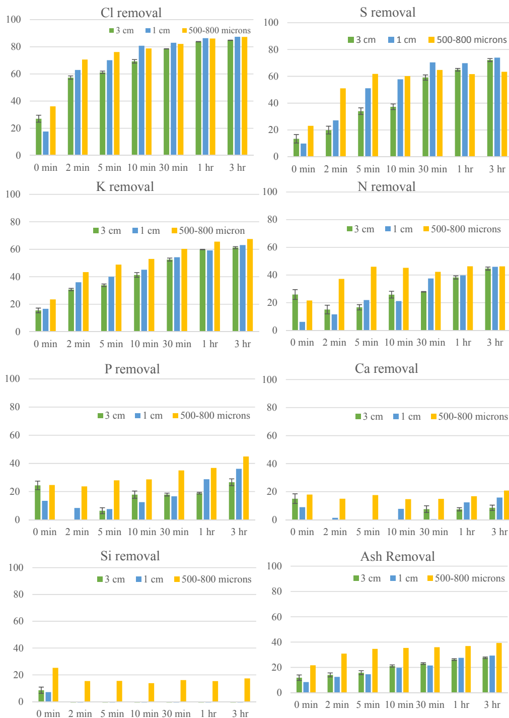
Fig. 2. The effect of time and size variation in the washing pre-treatment on the removal of (a) chlorine, (b) sulphur, (c) potassium, (d) nitrogen, (e) phosphorus, (f) calcium, (g) silicon, and (h) ash.
