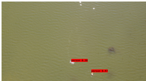
(a) Detection of one person (high confidence), and turbulent water next to another (lower confidence). Altitude: 37 m. Pitch: -80^\circ .
