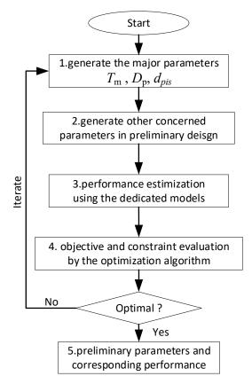
Figure 3. The flow chart of the preliminary design.
