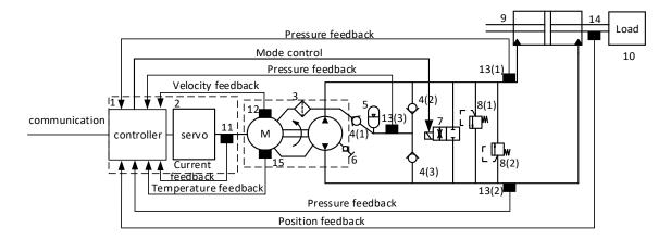
**Figure 1.** The schematics of the studied EHA: (1) Controller, (2) motor driver, (3) motor-pump unit, (4) check valves, (5) reservoir, (6) filling port, (7) solenoid valve, (8) relief valves, (9) cylinder, (10) load, (11) current sensor, (12) rotational speed sensor, (13) pressure sensors, (14) position sensor, (15) temperature sensor.
