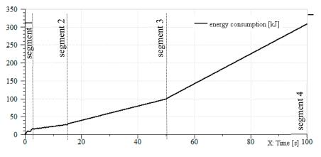
Figure 8. The energy consumption of the EHA.
