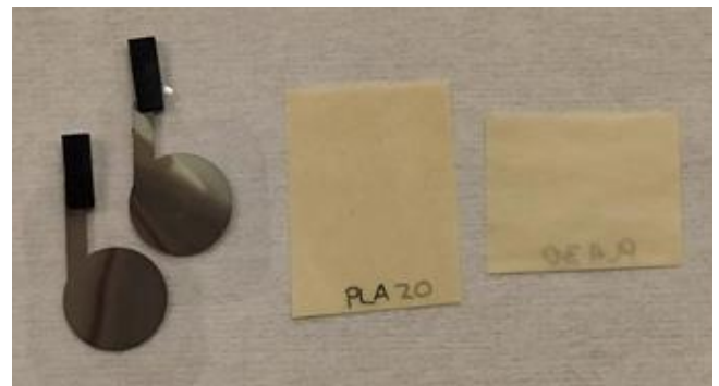
Fig. 4. Photograph of used evaporated silver electrodes on polyethylene terephthalate (PET) film and example of two in-house prepared PLA films.
