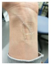
Fig. 5. IDE sensor attached to the skin.
