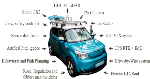
Fig. 7: EDI DbW car and its main components.
