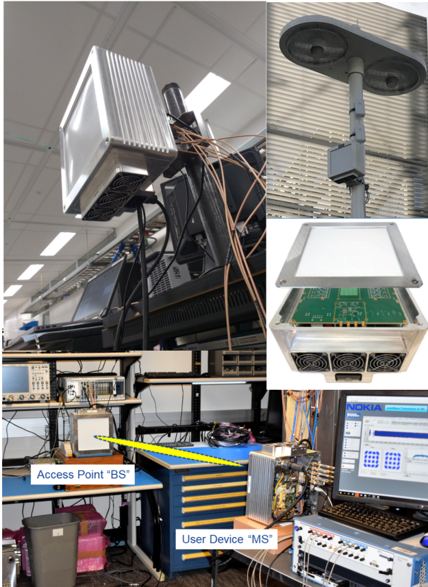
Fig. 2: Proof-of-Concept system [7]: the 93 GHz radio head and the access point - user device test link.
