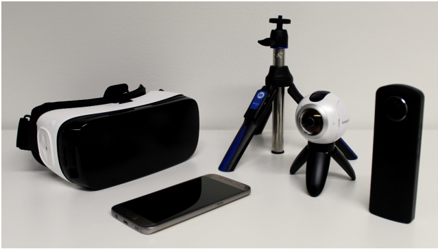
Figure 2: Equipment used in the study (from left to right): Samsung Gear VR headset, Samsung Galaxy S7 phone, Benro BK10 tripod, Samsung Gear 360 camera, and Ricoh Theta S camera.
