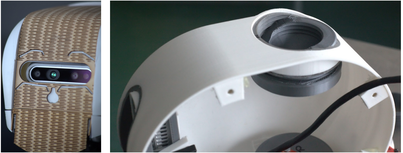
Fig. 5. Resulting designs of the parametric robot head. On the left a close-up image is shown of the wooden face structure with patterned flexibility, aimed towards a friendly look. On the right a close-up image is shown of the magnetic assembly points (white squares with holes) and the pluggable screw adapter for the microphone (grey). For a video, see https://youtu.be/2IJgnS1bGh0
