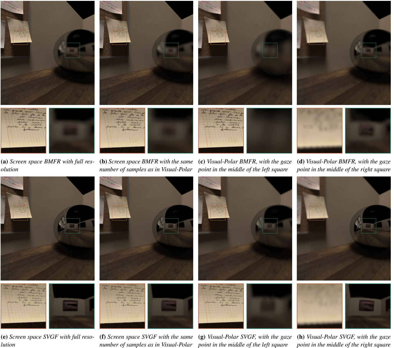
Figure 5: Example on how the denoisers can preserve reflections and details better when they are applied in the Visual-Polar space.
