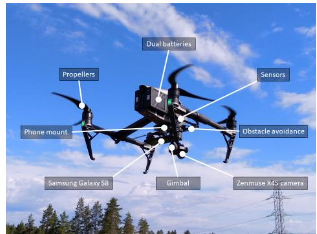
Figure 1. Measurement drone setup for data collection with a DJI Inspire 2 drone.
