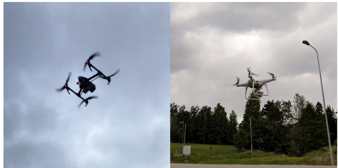
Fig. 2: Measurement drones. Inspire2 on the left and Phantom 4 Pro on the right.
