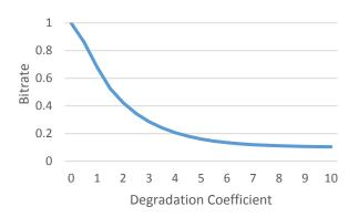
Fig 1. Bit rate of the encoded video relative to DC.
