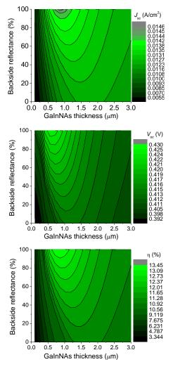
Fig. 4  $J_{sc}$ ,  $V_{oc}$  and  $\eta$  of a n-i-p solar cell as functions of reflectance of the diffuse reflector and GaInNAs thickness.
