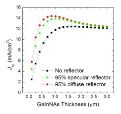
Fig. 2. Comparison of calculated  $J_{sc}$  vs. GaInNAs thickness for solar cells with and without reflectors. The simulation parameters for the cell are taken from [14]. The background doping level of the GaInNAs layer is  $2.2 \times 10^{16}$  cm<sup>-3</sup>.
